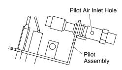
Figure 36 - Pilot Inlet Air Hole
